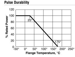
Limitation obtained by actual test with 0.01 duty continuous pulse repetition for TGHMV10R0JE, four times safety factor was considered. Please note this is not a specification, this is a typical
