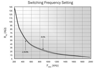
Figure 15. Switching Frequency vs. R<sub>FS</sub>
