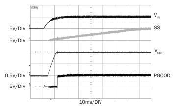
Figure 2. Start Up by V<sub>IN</sub>@4A
