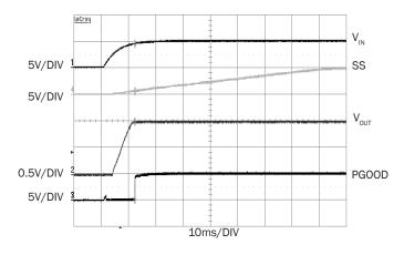
Figure 1. Start Up by  $V_{IN}$ @0A
