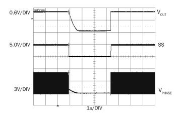
Figure 8. Thermal Shutdown Protection@0A
