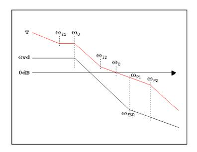
Figure 18. Asymptotic Diagrams of Power Stage and Loop Gain
