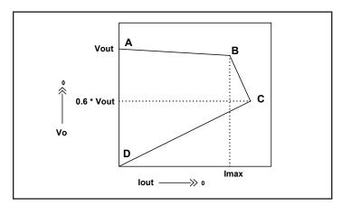
Figure 16. Over Current Protection Characteristic
