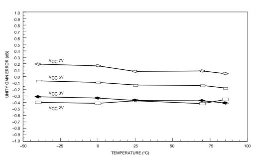
Figure 6. Unity Gain Error vs. Temperature and  $\rm V_{CC}$
