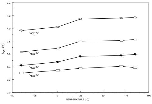
Figure 7.  $I_{CC}$  vs. Temperature and  $V_{CC}$
