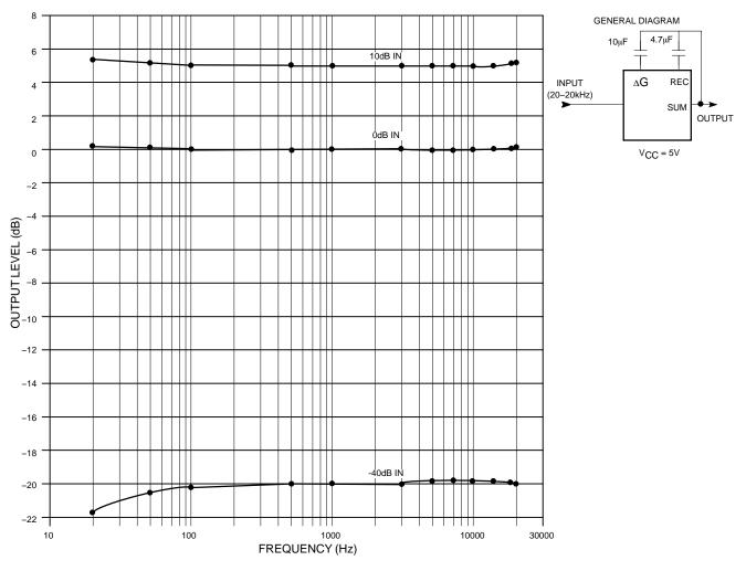
Figure 8. Compressor Output Frequency Response
