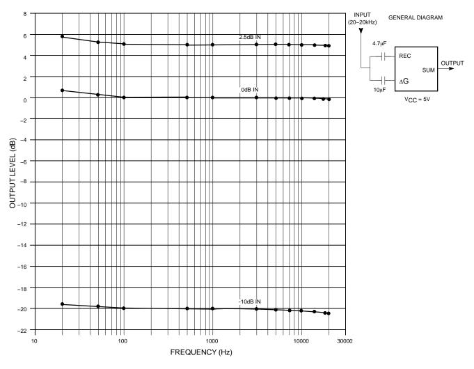
Figure 9. Expandor Output Frequency Response
