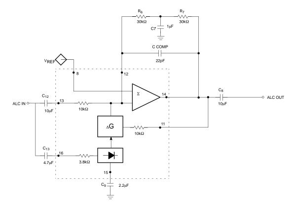
Figure 4. Typical ALC Configuration
