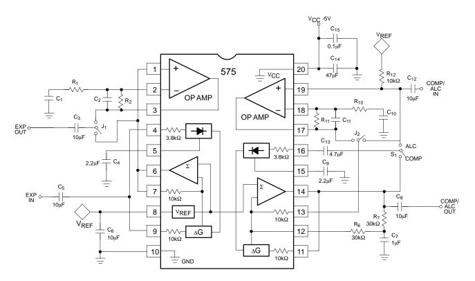
Figure 5. SA575 Low Voltage Expandor/Compressor/ALC Demo Board
