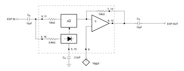
Figure 2. Typical Expandor Configuration
