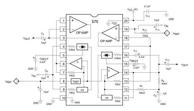
Figure 1. Block Diagram and Test Circuit
