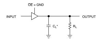
\*Includes all probe and jig capacitance.
