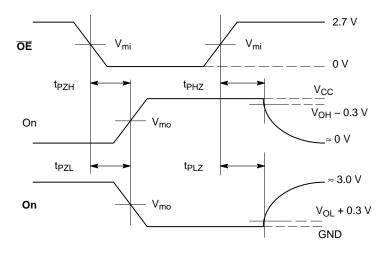
Figure 8. AC Output Enable and Disable Waveform
