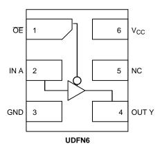
Figure 2. Pinout (Top View)
