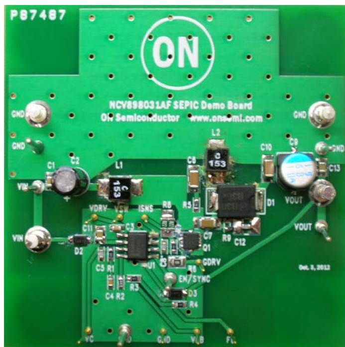
Figure 1. NCV898031 SEPIC Evaluation Board
