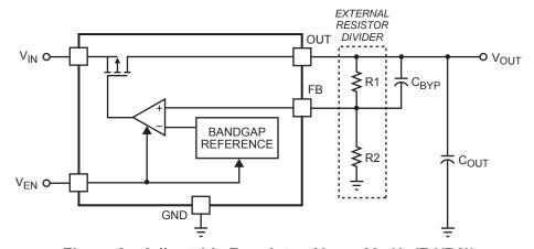
Figure 2—Adjustable Regulator:  $V_{OUT} = V_{FB}(1+(R1/R2))$
