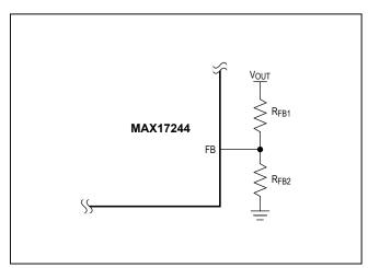
Figure 2. Adjustable Output-Voltage Setting
