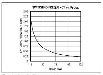
Figure 3. Switching Frequency vs. RFOSC
