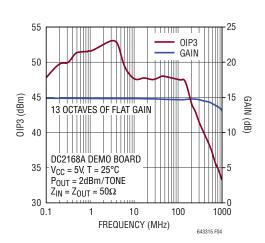
Figure 4. DC2168A Gain and OIP3 vs Frequency
