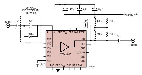
Figure 1. Test Circuit A Evaluation Circuit
