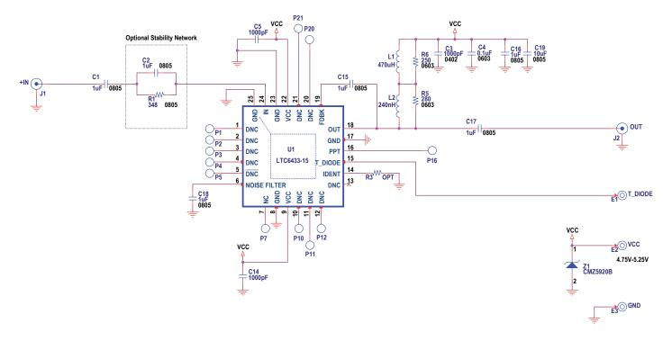
Figure 2. DC2168A Demo Board Schematic
