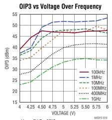
$\begin{aligned} &V_{CC}=5\text{V},\,T=25^{\circ}\text{C}\\ &P_{OUT}=2\text{dBm/TONE}\\ &f_{SPACE}=1\text{MHz}\\ &Z_{IN}=Z_{OUT}=50\Omega \end{aligned}$
