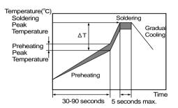
[Standard Conditions for Flow Soldering]
