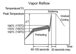
[Allowable Reflow Soldering Temperature and Time]
