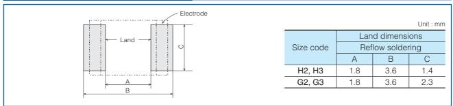
\* It is not warrantable that you can mount the capacitor without trouble under all the mounting condition when "Recommender for Land dimensions" is adopted.
