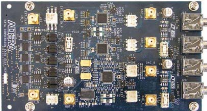
Figure 2. Cyclone III Data Conversion HSMC
