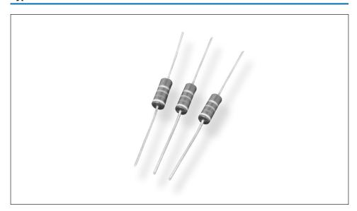
The CBT series of resistors is constructed utilising solid carbon composition, which is the traditional medium for absorbing high energy pulses, in cases of high inrush current. These resistors have evolved over many years to have excellent pulse withstand capabilities, whilst remaining very stable. These improved characteristics have been achieved by prudent selection of materials of optimum physical properties and by advances in the manufacturing process.
