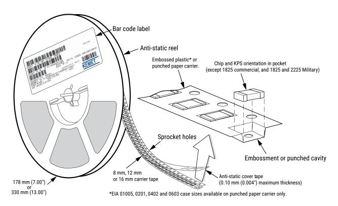
Table 6 - Carrier Tape Configuration, Embossed Plastic & Punched Paper (mm)
