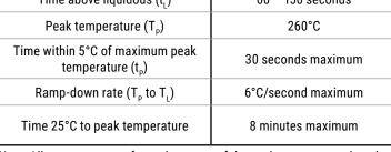
Note: All temperatures refer to the center of the package, measured on the capacitor body surface that is facing up during assembly reflow.
