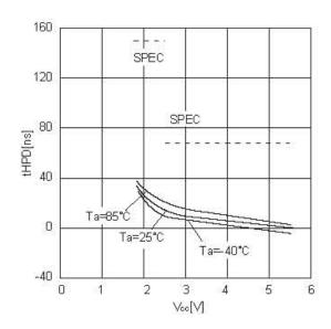
Figure 28. Time from HOLD to output High-Z tHOZ
