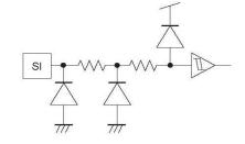
Figure 58. SI input equivalent circuit
