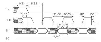
Figure 1. Input timing
