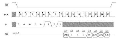
Figure 42. Status register read command (BR25L080/160/320/640-W)
