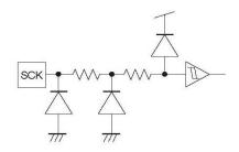
Figure 57. SCK input equivalent circuit
