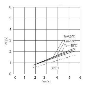
Figure 5. "L" input voltage VIL
