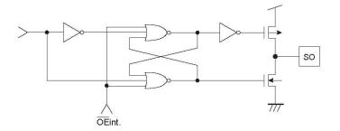
Figure 55. SO output equivalent circuit
