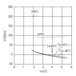
Figure 19. CS setup time tCSS
