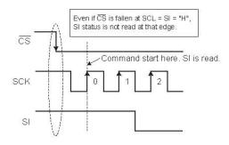
Figure 43. Operating timing
