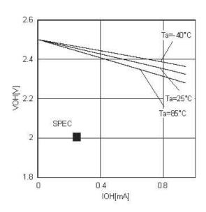
Figure 9. "H" output voltage VOH-IOH(Vcc=2.5V)
