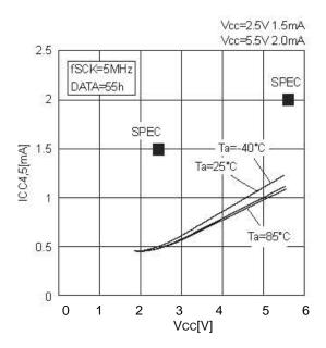
Figure 12. Current consumption at WRITE operation ICC1,2,3 (WRITE,PAGE WRITE,WRSR,fSCK=5MHz) BR25L010-W,BR25L020-W,BR25L040-W
