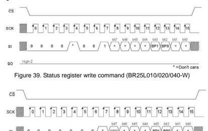
Figure 40. Status register write command (BR25L080/160/320/640-W)
