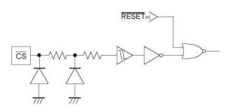
Figure 56. CS input equivalent circuit
