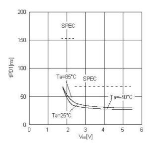
Figure 23. Data output delay time tPD1(CL=100pF)
