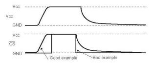
Figure 61. CS timing at power ON/OFF
