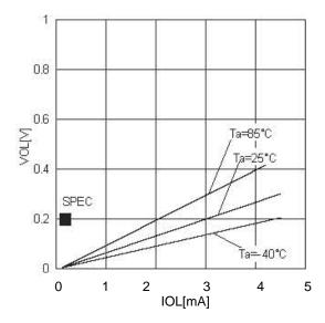
Figure 6. "L" output voltage VOL-IOL(Vcc=1.8V)
