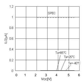
Figure 11. Output leak current ILO(SO)
