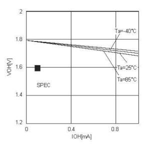
Figure 7. "H" output voltage VOH-IOH (Vcc=1.8V)
