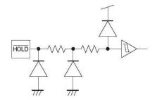
Figure 59. HOLD input equivalent circuit
