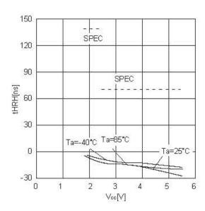
Figure 27. HOLD release hold time tHRH
