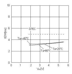
Figure 32. Write cycle time tE/W
