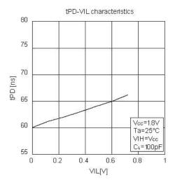
Figure 53. VIL dependency of data output delay time
