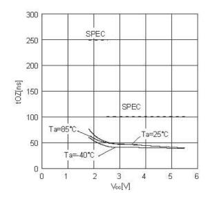
Figure 24. Data output delay time tPD2(CL=30pF)
