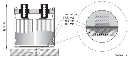
Dimensions and weights for heat sink mounting:
