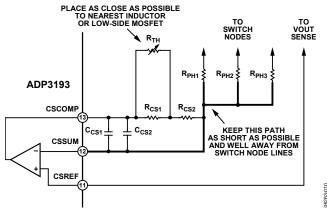
Figure 11. Temperature Compensation Circuit Values
