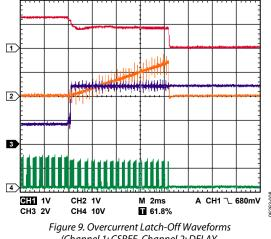
(Channel 1: CSREF, Channel 2: DELAY, Channel 3: COMP, Channel 4: Phase 1 Switch Node)
