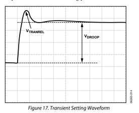
Because the ADP3193 turns off all of the phases (switches inductors to ground), no ripple voltage is present during load release. Therefore, the user does not have to add headroom for ripple, which allows load release  $V_{\text{TRANREL}}$  to be larger than  $V_{\text{TRAN1}}$  by the amount of ripple, and still meet specifications.
