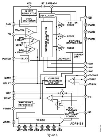
The ADP3193 has a built-in shunt regulator that allows the part to be connected to the 12 V system supply through a series resistor.
