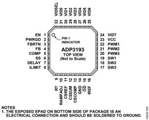
Figure 5. Pin Configuration
