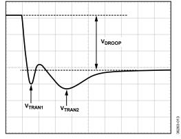
Figure 16. Transient Setting Waveform
