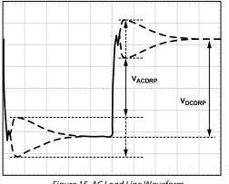
Figure 15. AC Load Line Waveform
