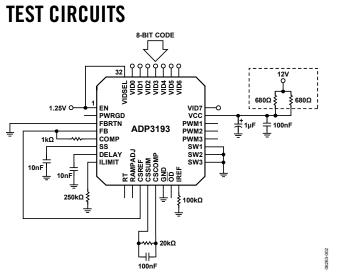
Figure 2. Closed-Loop Output Voltage Accuracy
