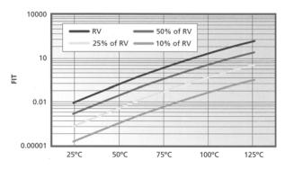
Component type: Testing Location: Results based on: 0805 (COG/NP0 and X7R) Syfer reliability test department 16,622,000 component test hours
